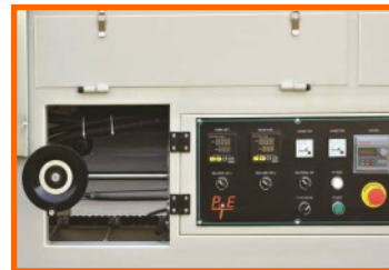
Lower IR Lamp raising and lowering adjustment.
