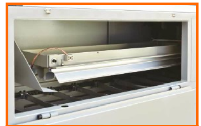
Upper IR Lamp with full-access door open.
