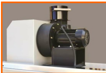
Exhaust for removal of humidified air.
