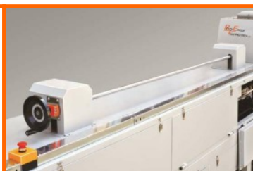
Upper IR Lamp raising and lowering with digital readout.
