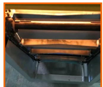
Outfeed of IR Dryer with jog button for easy cleaning and maintenance.
