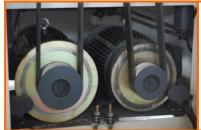
Pneumatic disc brake on all main drive motors.
