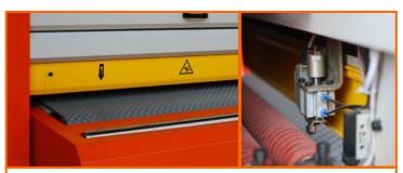
Automatic digital electronic measuring device for panel thickness complete with manual fine adjustment knob; adjustable in 0.01mm increments.
