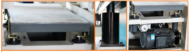
Heavy duty granite surface table, strong and robust without any deflection for a superior finished product. Massive base-frame welded from plate and structural steel and a removable access panels for easy maintenance. Positioning of granite work table through four heavy duty chain driven precision machined lifting screws.
