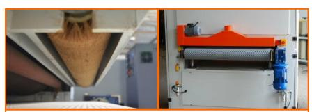
Independent brush cleaning and vacuum dust extraction comes **standard** on all models for a cleaner finished product.
