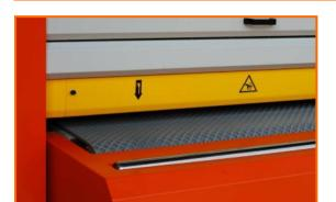
Automatic thickness setup with digital position controller for precise dimension settings and digital readout with micro adjustment. Over-thickness protection comes **standard** on all models. Adjustable material from 2mm - 100mm.
