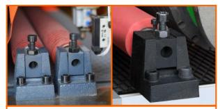
(2) grooved spring-loaded rubberized pressure rollers for part hold-down positioned on the 1st head and (1) grooved roller positioned between the 1st and 2nd head. A solid rubberized pressure roller positioned behind the 2nd head.
