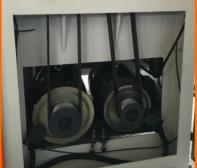
Both the 1st and 2nd head motors are Star-Delta starting or "Soft-starting" for low power consumption during start-up. This is a **MUST HAVE** for any shop with an Electric Demand Meter.
